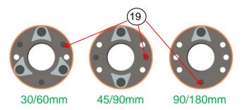
The control wheel comes with threaded holes which are in a circular alignment. The cams (17) must be screwed (18) into these holes by always keeping the gap you can see in the different pictures. The hole that is marked with X is always in use. For the distances at the Skater 14414707 the cams are screwed in both side's front and back (19) of the control wheel!
