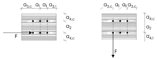
For screws in the edge surface, a<sub>1</sub> and a<sub>3</sub> are parallel to the CLT plane face, a<sub>2</sub> and a<sub>4</sub> perpendicular to CLT plane face.
